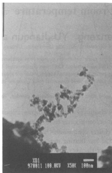
Fig. 2. TEM picture of CuO nanometer powder.
