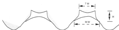
Fig. 5. Measurements used to characterize the two-peaked glume cell, type 22IIIAb. TW: top width; MW: width at the point where the glume projection (hair) attaches to the base; H: height of each hair.
