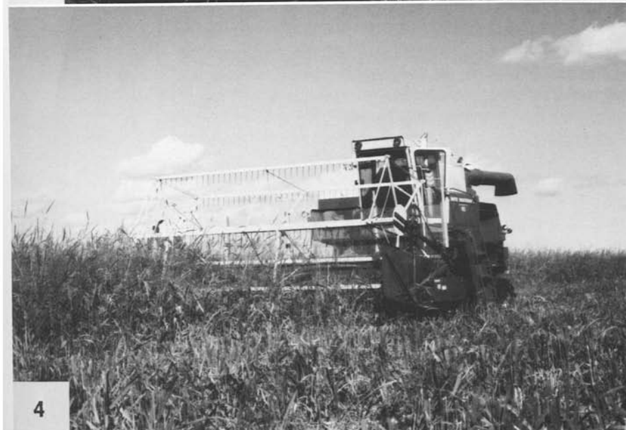
Fig. 3-4. Wildrice. Fig. 3. Example of a wildrice harvester that can make repeated trips through a cultivated stand of shatter-susceptible wildrice without destroying the plants. Repeat harvests of shatter-susceptible varieties are necessary to collect kernels as they mature. Fig. 4. Retention of mature seed on shatter-resistant cultivars permits once-over harvest with rice ( Oryza sativa ) combines.
