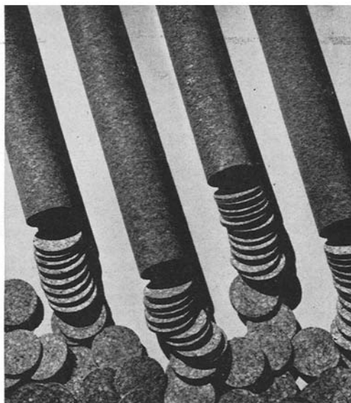
FIG. 7 (Left). Cork is an excellent low temperature insulation material.
