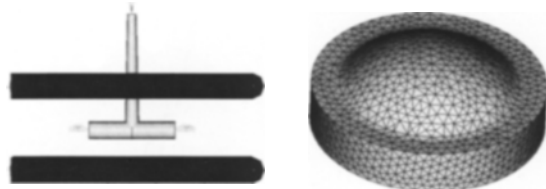
(a) The finite model of the mold (b) The finite model of the lens
