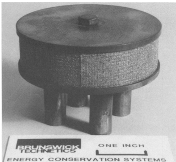
Fig. 4. Test apparatus: specimen holding fixture shown with cylindrical specimen.
