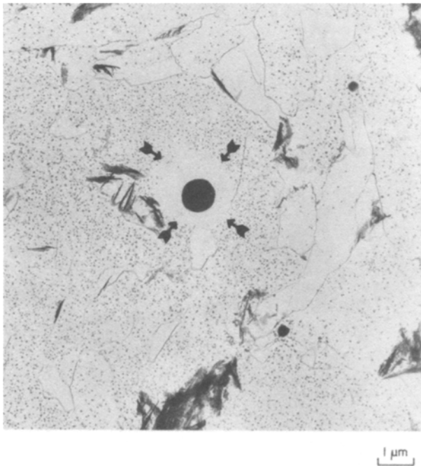
Fig. 19. TEM micrograph showing the presence of small \alpha -MnS inclusions around a larger oxide particle.
