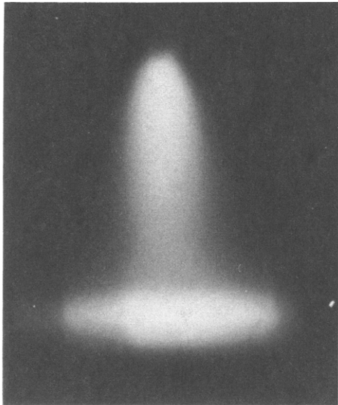
Fig. 10—Monochromatic photograph of a 125 A arc on the high sulfur 304 steel (W156) at a manganese characteristic wavelength (argon shielding gas).
