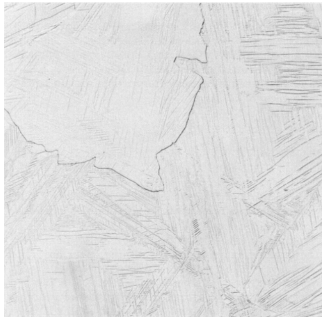
Fig. 7—V-10.1 at. pct O alloy quenched from 240°C. Single-phase \alpha' . Magnification 281 times.
