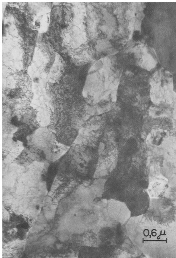
Fig. 1—Microstructure of "acicular ferrite" HSLA Steel, magnified 17,600 times.
