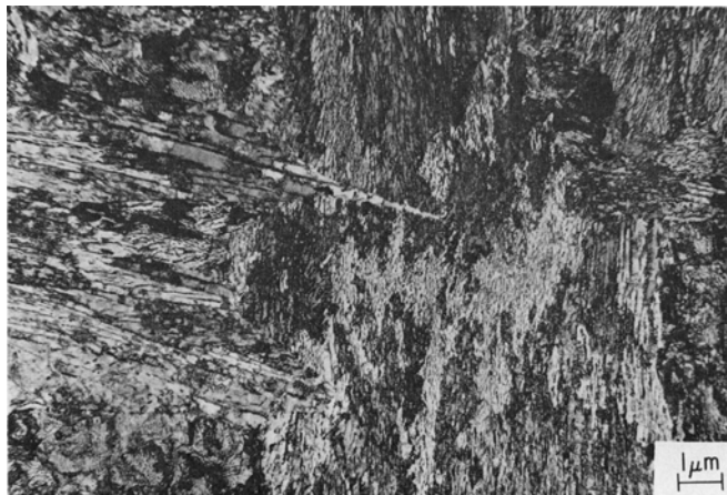
Fig. 6—Transmission electron micrograph of upper bainite in as-patented steel wire.
