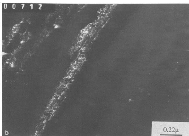
Fig. 6— M_2C carbides at a lath boundary in alloy M(M2) after 100 min at 600 °C. (a) TEM, bright-field image and (b) TEM dark-field image using (020)_{M_2C} reflection.
