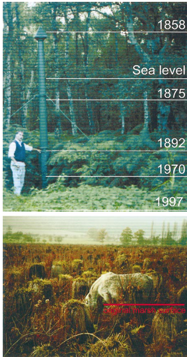
Fig. 1. Upper: The Holme Post at Holme, England in July 1997. The dates are the surface elevation at that time. The post was sunk into a clay layer in 1848, and the height of the surface layer determined since. The surface of the peat was originally above sea level (marked), but the peat is now 2 m below sea level (photograph by the author). Lower: Horse grazing in the La Grand-Mare Marais-Vernier, Normandy, France. The Marais-Vernier is part of the Brotonne Regional Natural Park. The top of the tussocks was the surface of the marsh before drainage. Photograph courtesy Dr. J. Pokorny, Trebon, Czech Republic.
