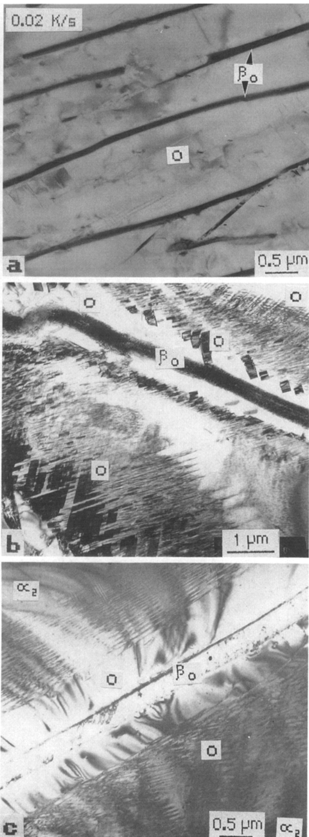
Fig. 11—Lath structures obtained in specimens slow furnace cooled from \beta at 0.02 K/s: (a) O + \beta_0 structure, (b) O laths with multivariant plate O in the core and monolithic O at periphery, and (c) laths with \alpha_2 in the core and plate O and monolithic O.
