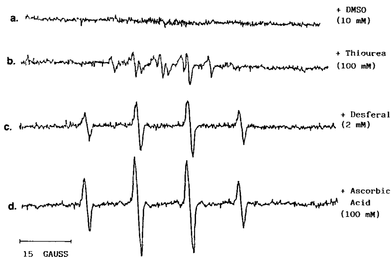
Fig. 3. ESR spectra recorded 1 min after mixing in a Tris buffer solution (pH 7.4) of 2 mM \text{Cr}^{6+} , 2 mM NADPH, 2 mM \text{H}_2\text{O}_2 , 12 U/mL GRx, and 500 mM DMPO with (a) 10 mM DMSO (b) 100 mM Thiourea, (c) 2 mM Desferal, and (d) 100 mM ascorbic acid. Spectrometer settings were same as Fig. 1.
