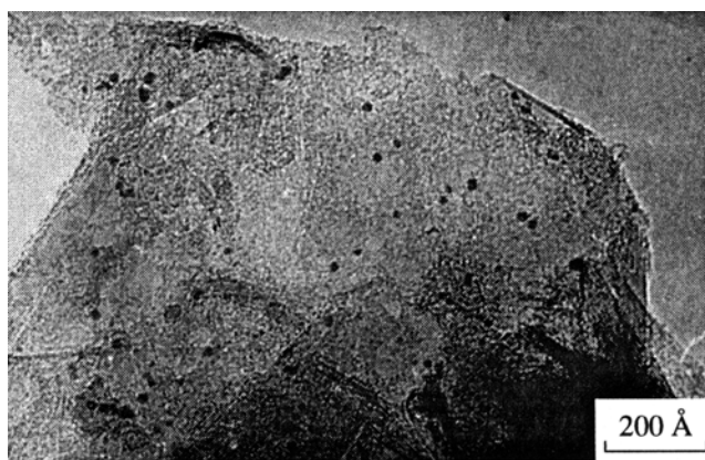
Fig. 6. A HREM pattern of the sample of Sibunit saturated by Pd(II) compounds from a solution of PHC.
