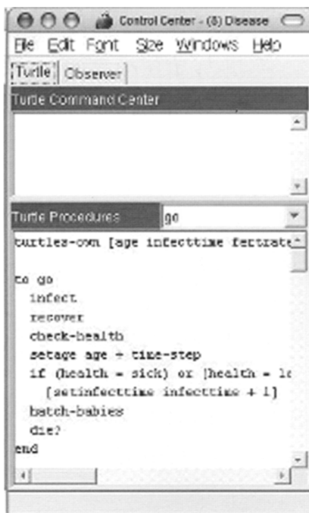
Figure 1. A simple epidemic model in the current version of StarLogo. A section of code for the model is seen on the left, while the run time view is seen below.
