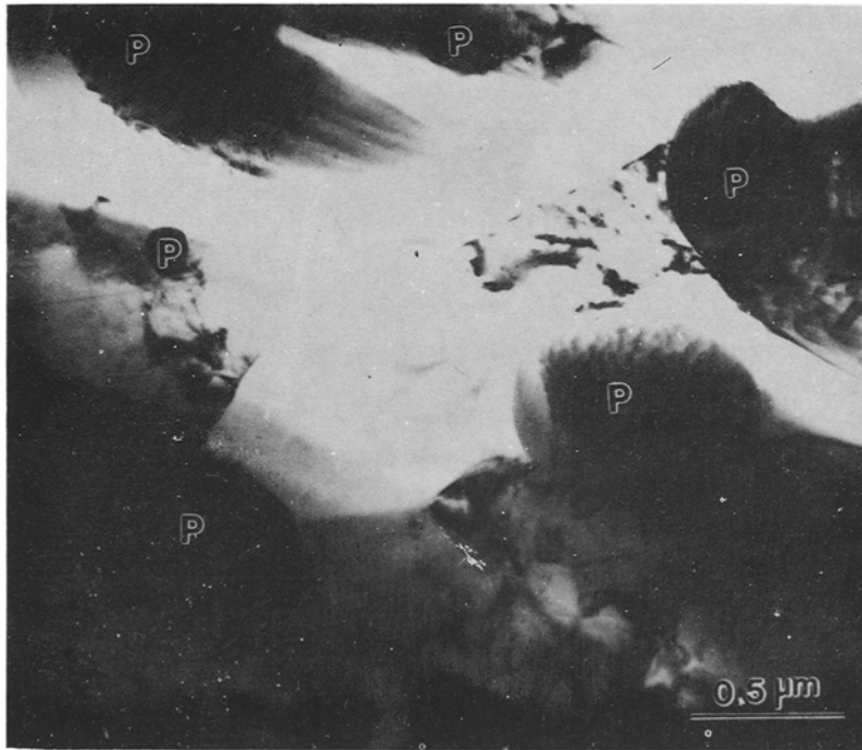
Figure 15. TEM micrograph of microstructure of XD Al/TiC composite after room-temperature tension test (area close to fracture surface). Regions around the particles are misoriented with respect to each other and hence the contrasts are different (Fine et al 1993).
