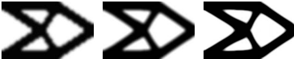
Figure 18. The cantilever beam with material interpolation function (5) q = 6 . The parameters H = 1/15 , R = 0.1 and \tilde{c}_2 = 5.0 \cdot 10^{-4} are used and the number of optimization iterations are 65,61 and 181 respectively
