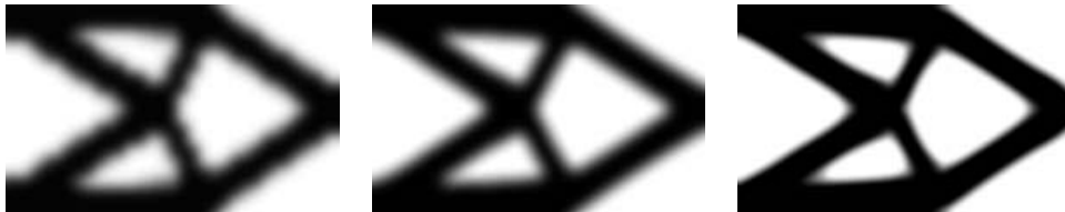
Figure 19. The cantilever beam with material interpolation function (4) q = 3 . The parameters H = 1/10 , R = 0.15 and \tilde{c}_2 = 7.5 \cdot 10^{-4} are used and the number of optimization iterations are 55,543 and 641 respectively
