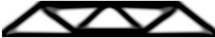
Figure 13. The MBB beam ( M_5 ) with filtered sensitivities
