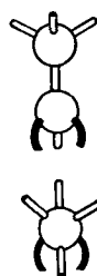
Fig. 8. - Positions of minimum energy of the single bonds of a carbon atom singly linked to a double-bonded one (side and end views).
