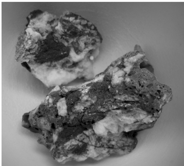
Fig. 1. A photograph of natural gas hydrate sample collected at Site 1249 on Leg 204 in Oregon offshore. The white parts represent natural gas hydrates.
