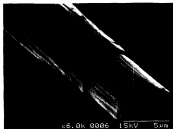
Fig. 2. Scanning electron micrograph of the SiC-coated carbon fiber.
