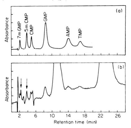
**Figure 5.** HPLC of deoxynucleotide monophsophates. The solvent conditions and other experimental details were as described under Materials and methods. A. Separation of standards.
