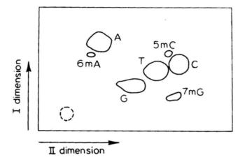
**Figure 4.** Separation of deoxynucleotide monophosphates on two dimensional TLC. Diagrammatic representation of observed separation of standard dNMPs following chromatography on cellulose TLC plates using Isobutyric acid: water: NH<sub>4</sub>OH (66:20: 1,  $\nu/\nu$ ) in the first dimension and saturated (NH<sub>4</sub>)<sub>2</sub>SO<sub>4</sub>: in the second dimension.
