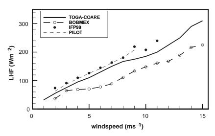
Figure 4. Mean variation of the latent heat flux with wind speed observed during TOGA-COARE, BOBMEX, IFP99 and BOBMEX-Pilot experiments.
