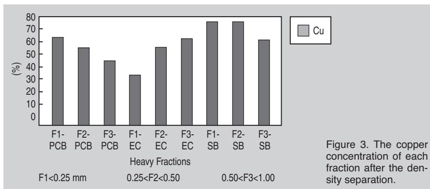
Figure 3. The copper concentration of each fraction after the density separation.
