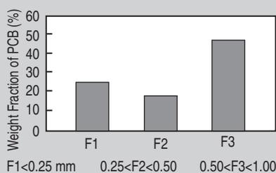
Figure 1. The results of size classification from complete printed circuit boards (PCB) after comminution in a knife mill.
