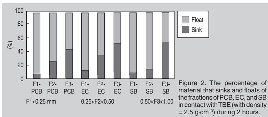
Figure 2. The percentage of material that sinks and floats of the fractions of PCB, EC, and SB in contact with TBE (with density = 2.5 g·cm<sup>-3</sup>) during 2 hours.
