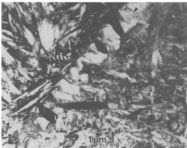
Fig. 6—TEM micrograph of 60 °C/s Gleeble specimen. Arrows indicate position of grain boundary.
