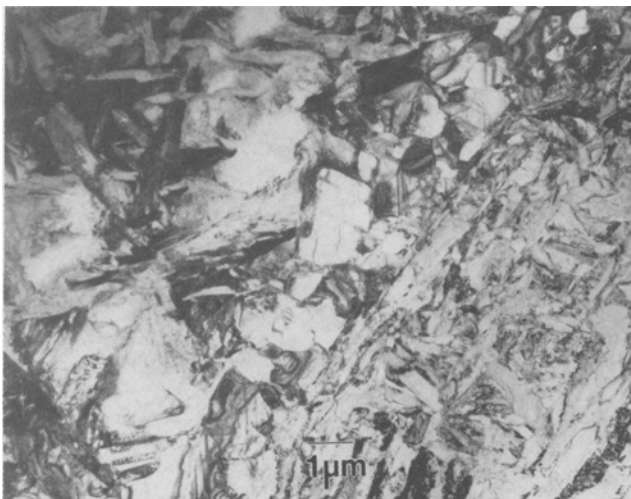
Fig. 16—TEM micrograph of fusion zone microstructure in GTA weld metal. Intragranular acicular \alpha_2 laths and grain boundary equiaxed \alpha_2 are both present.
