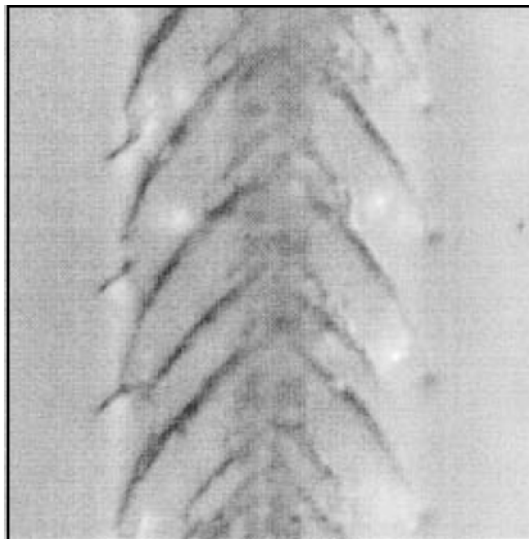
Figure 13—Optical image of a scratch made by the face of a cube corner. The sample surface is tilted 10^\circ .
