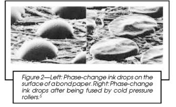
ing paper and transparencies. The hot melt ink composition may not obtain sufficient clarity and adhesive properties if the bisamide wax is too small a fraction of the total wax content. On the other hand, the melting point of the hot melt ink composition may become difficult to control if too much bisamide wax is used. Bisamide wax is usually present in hot melt ink formulation in an amount of  $10~{\rm to}~50\%$  by weight.^27
