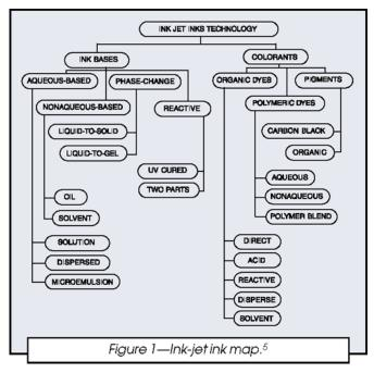
which is very important for continuous ink jet, is not an issue for DOD technology. Therefore, inks for CIJ are more demanding than the DOD inks. Many different types of inks have been developed and used in ink-jet applications (*Figure* 1).
