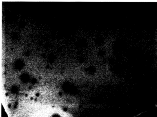
Fig. 4. TEM scan of a thin film, cast from DMF, of a 5/95 blend of PMMA ionomer (6 mol %)/PMMA [Tsou, 1997].
