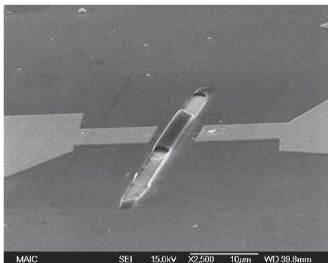
Fig. 3. Scanning electron microscopy of ZnO nanorod with integrated microchannel (4- \mu m width).
