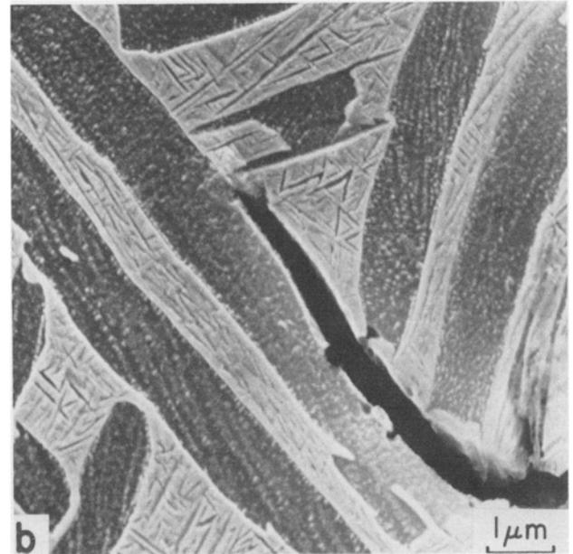
Fig. 4—Fatigue fracture of Ti-6Al-2Sn-4Zr-6Mo tested at  $R = 0.1$  and 20 Hz in dry air: (a)  $\alpha/\beta$  processed material,  $\Delta K = 4.5 \text{ MN/m}^{3/2}$ ,  $da/dN = 2.5 \times 10^{-6} \text{ mm/cycle}$ ; (b)  $\beta$  processed material,  $\Delta K = 5.0 \text{ MN/m}^{3/2}$ ,  $da/dN = 2.5 \times 10^{-4} \text{ mm/cycle}$ .
