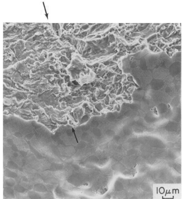
Fig. 3—Fracture surface of a fracture toughness specimen of Ti-6Al-4V in a STOA condition. Note the transition region (arrows) between the fatigue precrack and the tensile fast-fracture regions.
