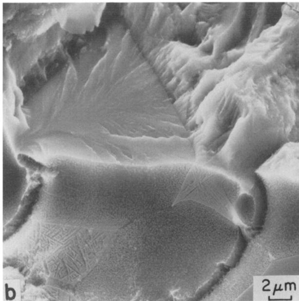
Fig. 2—Fatigue fracture of Ti-6Al-4V in a recrystallization annealed condition tested at  $R = 0.1$  and 20 Hz in dry air,  $\Delta K = 9.9 \text{ MN/m}^{3/2}$ ,  $da/dN = 2.5 \times 10^{-6} \text{ mm/cycle}$ .
