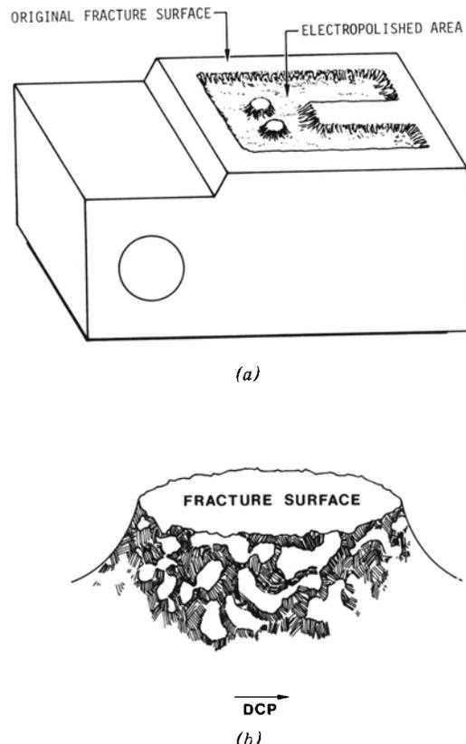
Fig. 1—Schematic of methods of stopping off areas to be examined: (a) overall specimen; (b) details of a typical spot.
