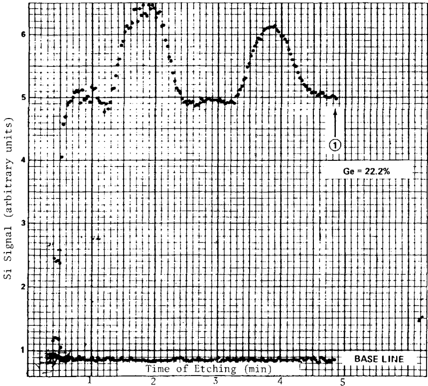
Figure 4. Auger Profile of the Si Content in Several Layers of an Alternating, Multilayer Film with X=0.22 . The Ge content was determined by direct measurement of the Ge signal at several selected points.
