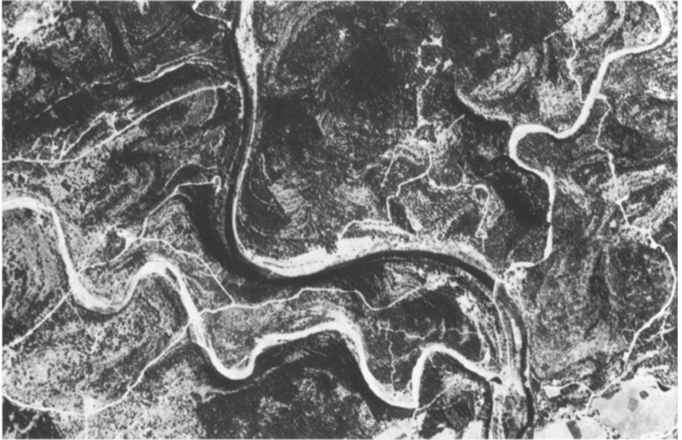
Figure 24. NASA infrared aircraft imagery of the Guadalupe River canyon below Canyon Dam and upstream from New Braunfels, Texas. The bright response areas are alluvium and scour in tributary stream valleys resulting from flooding of May 11 and 12, 1972. Frame depicts a scene 3 \times 5 km.
