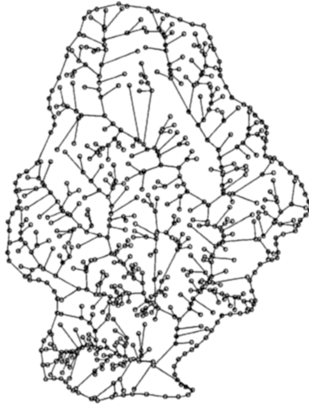
Figure 14. CALCOMP plot of drainage network data used for detecting machine or operator errors encountered in the digitizing operation.
