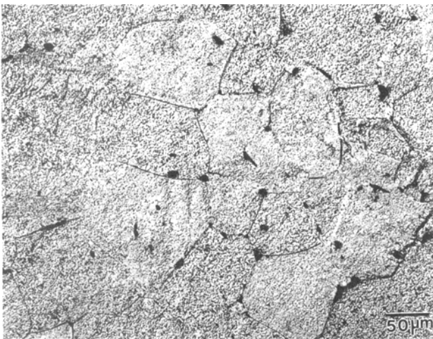
Fig. 5—Optical micrograph showing equiaxed grain morphology of a spray-deposited Al-Li sample taken from experiment 1, heat-treated at 400 °C for 100 min.
