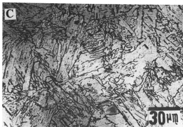
Fig. 2—Microstructure of alloy T1 transformed at 550 °C for (a) 3 sec (granular bainite regions are shown with arrows), (b) 20 sec (part of the ferrite plates have coalesced so that some of the bainite packets develop a massive contour), and (c) 300 sec (most of the original bainite packets develop a massive contour).
