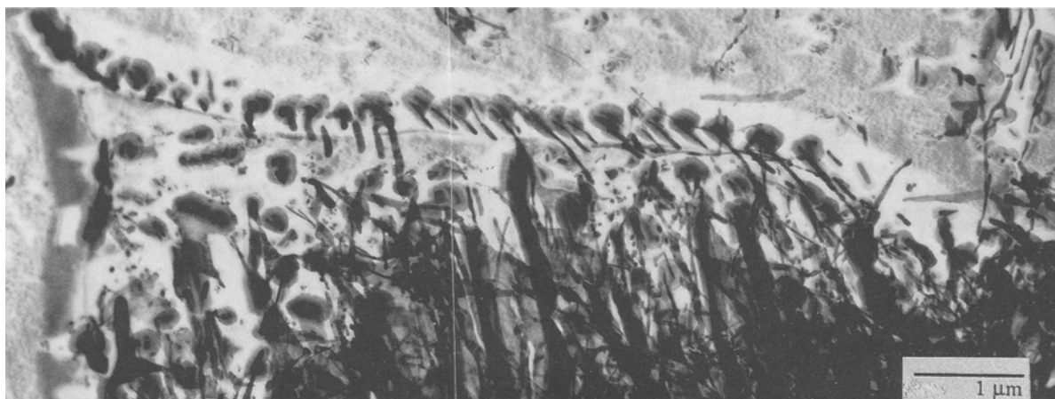
Fig. 13—Replication micrograph of fibers developing from carbides nucleated at an \alpha:\gamma boundary. Reacted 200 s at 700 °C.
