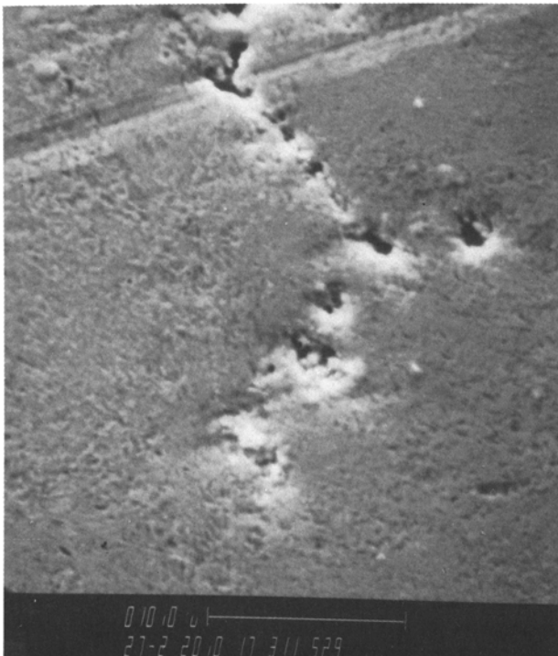
Fig. 6—Porosity development in U-10Zr fuel at \sim 0.8 at. pct burnup [right, hot center of pin and, left, cooler fuel toward pin surface (SEM, SE)].
