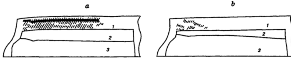
Fig. 4. Damage zones for solid (a) and porous (b) shields: 1) chamber; 2) shield; 3) detonation products.
