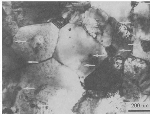
Fig. 1—Representative TEM microstructure of the Fe-10 pct Cu (700 °C HIP) specimen. Likely copper grains, based on numerous dark-field images taken in similar foils, are indicated by arrows.
