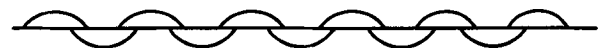
Fig. 13—A schematic side view of an array of semicoherent grain boundary allotriomorphs (say M_{23}B_3C_3 ) which acts to prevent nucleation of a subsequent reaction product.
