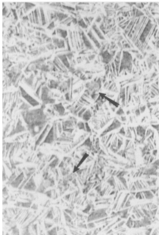
Fig. 8—Cinematograph micrographs representing the critical cooling rate for the Fe-0.8 pct C alloy (near data points G and H in Fig. 7). This series shows the limit of growth of the pearlite nodules (arrow) followed by the formation of martensite. Magnification about 440 times.
