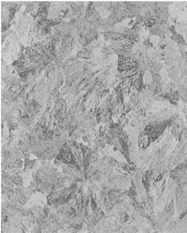
Fig. 7—A series of photomicrographs representing the structures produced at eight different cooling rates for the Fe-0.8 pct alloy. The letters correspond to the lettered data points in Fig. 6. Picral. Magnification 200 times.
