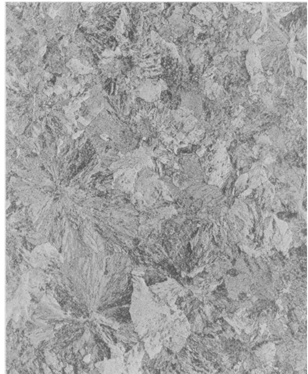
Fig. 7—A series of photomicrographs representing the structures produced at eight different cooling rates for the Fe-0.8 pct alloy. The letters correspond to the lettered data points in Fig. 6. Picral. Magnification 200 times.
