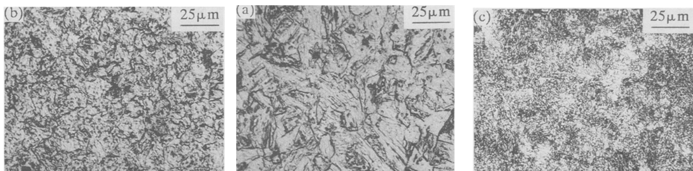
Fig. 2—Optical micrographs of Fe-13Mn-3Al alloy: (a) as-rolled, (b) ( \alpha + \gamma ) and \gamma cycled, and (c) lower ( \alpha + \gamma ) region tempered.
