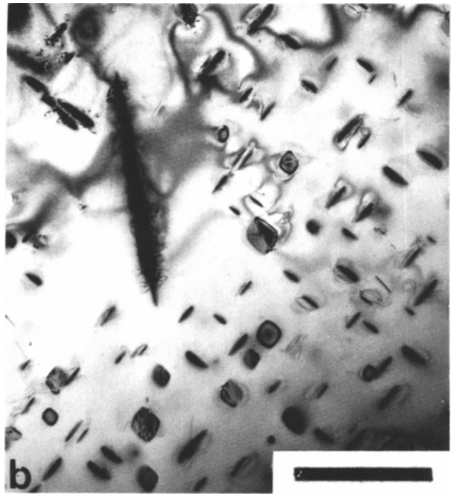
Fig. 8—Specimen aged at 1073 K (800°C) for 4 h; (a) bright field image showing alignment of particles (indicated by an arrow) leading to the formation of Widmanstaetten \beta phase as shown in (b). Foil orientation in (b) is [001]. Marker denotes 0.5 \mu\text{m} .
