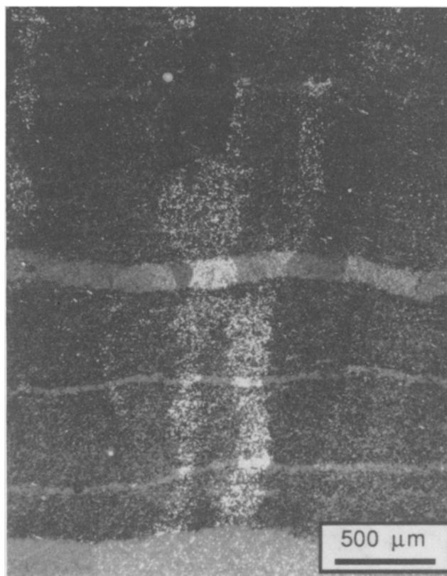
Fig. 15—Optical micrograph of the preform entrance region of etch-pitted SAFFIL alumina-fiber-reinforced 99.9 pct pure aluminum matrix composite viewed under crossed polarizers in the optical microscope. Large columnar grains are visible (in white) in this region. The preform entrance is at the bottom of the figure, and infiltration occurred upward. Horizontal striations are due to delamination of the preform.
