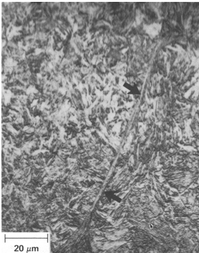
Fig. 6—Microstructure of specimen 1P, showing what appears to be a thin zone of modified material (arrows) at a powder particle interface. The structure of the particle interior is unchanged.
