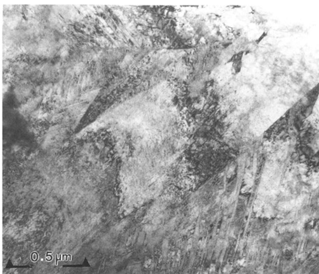
Fig. 2—Bright-field images of as-quenched and cryogenically treated steel showing martensite plates and twins.
