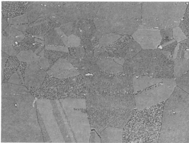
Fig. 1—Microstructure of the Udimet 700 alloy. Magnification 160 times.
