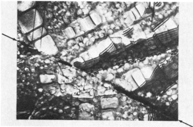
Fig. 15—Concentration of plastic deformation in coherent annealing twin boundary (arrows). Magnification 27,500 times.
