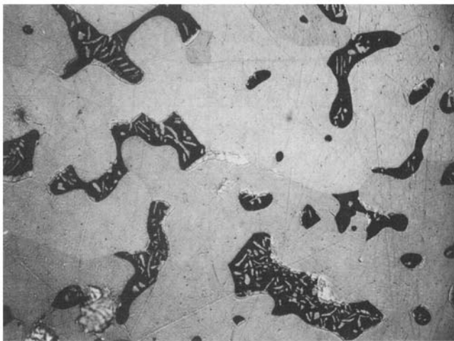
Fig. 2—18 at. pct Pt annealed at 1150^\circ\text{C} for three weeks. Nb 3 Pt (light) matrix containing \alpha -Nb (dark) globules in which precipitation of Nb 3 Pt has occurred during annealing. Magnification 296 times.
