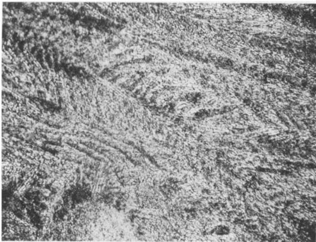
Fig. 5—45 at. pct Pt "as-cast" fine eutectic of \sigma + Nb_{1-x}Pt_{1+x} . Magnification 296 times.
