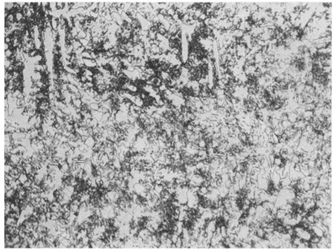
Fig. 6—55 at. pct Pt annealed at 1690 °C for six hours. Metastable primary Nb_{1-x}Pt_{1+x} dendrites and an unresolved fine structure of Nb_{1-x}Pt_{1+x} + NbPt_2 produced by decomposition of prior \alpha' -Pt. Magnification 296 times.
