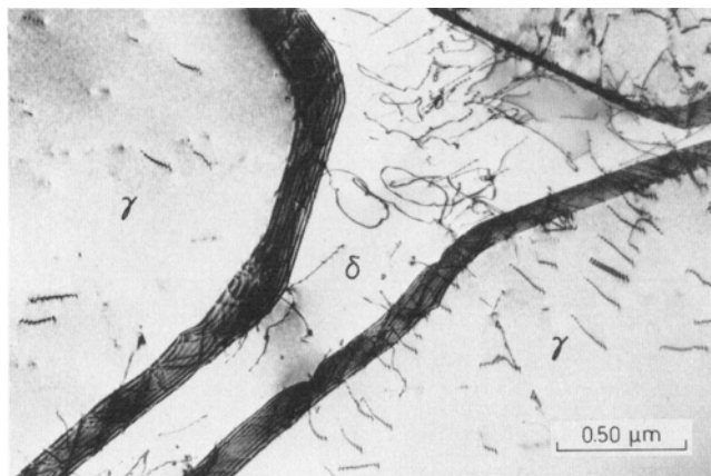
Fig. 9—Thin foil micrograph illustrating vermicular ferrite ( \delta ) and austenite ( \gamma ) in the same weld as in Fig. 4(a).
