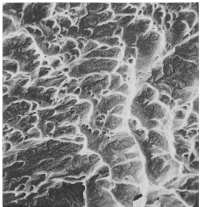
Fig. 3—Stereo pair of scanning electron micrographs of fracture surface showing that the dimples occur on many roughly parallel planes.
